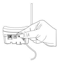
3. Place the AC Adapter cord around the strain relief.
